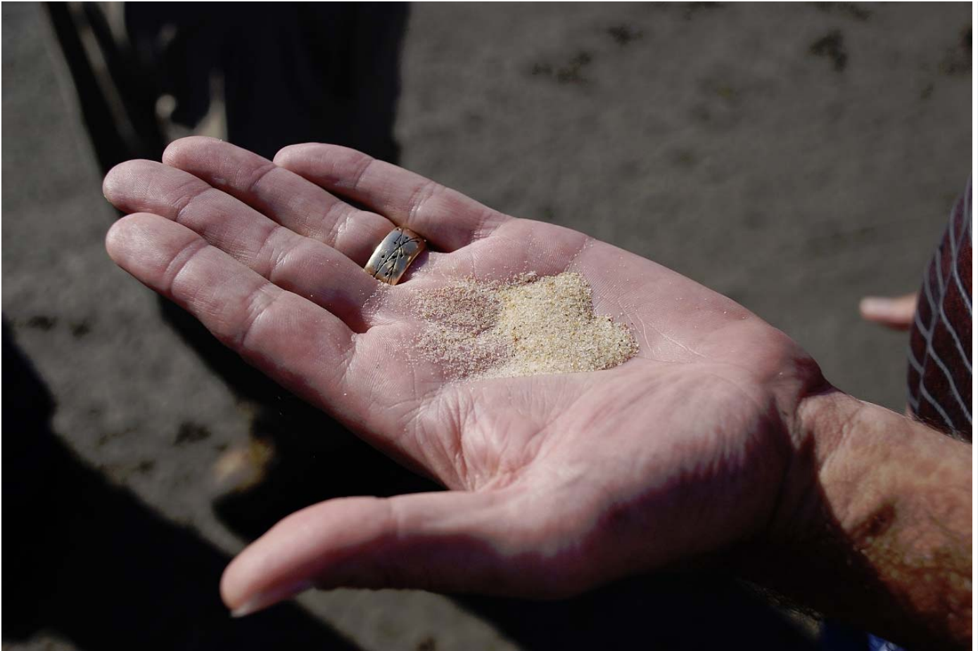
Sand is mixed with chemicals and water to prop the fractures open, allowing oil and gas to flow to the wellbore and then to the surface. U.S. Geological Survey/photo courtesy of Bill Cunningham.
